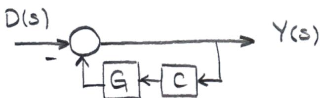
$$Y(s) = \frac{L(s)}{1 + L(s)} D(s) \quad \left[ \approx \frac{\text{forward}}{\text{loop ratio}} \right]$$
